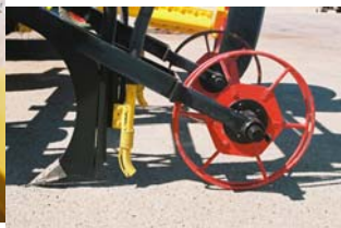
▼ Tyne assembly with spring steel press wheel.
