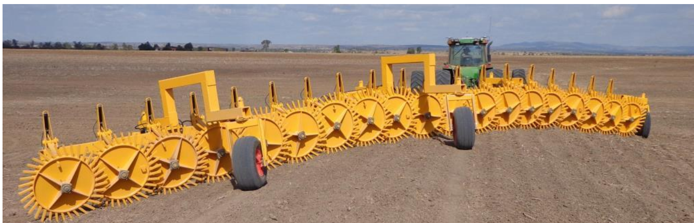
▲ Large Rakes are now hinged every fifth pin wheel to hug contour banks and uneven ground. Jumbo aircraft tyres are fitted to avoid punctures. NB Special 19 wheel pictured, new 18 wheel models have three U frame arches.
