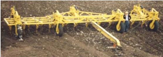
▲ Multiworker Chisel Plough for conventional farming in tough conditions.
