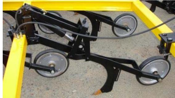
▲ Multiplanter tine assembly. Press wheel depth controlled seed tube and digging tip
