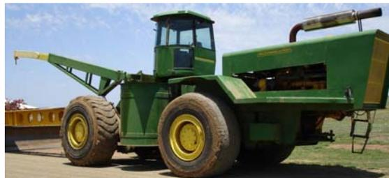
▲ Homemade tractor with Cat D9 engine and 90° swing around cab.
