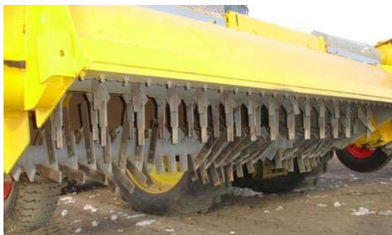
▲ Cotton Mulcher Blades. The 5" diameter flail shaft from the new design runs 60 blades, 2" apart through a 60 slotted comb.
