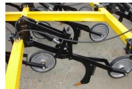
◀ Parallelogram controlled tyne assembly with 2" spear tip.
